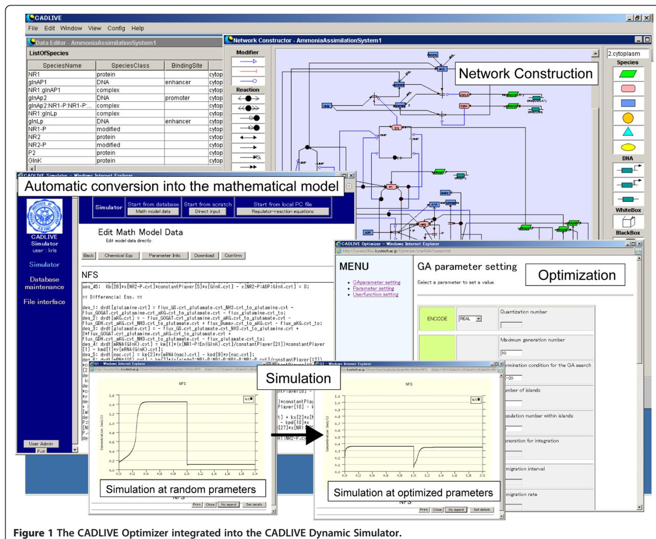
**Figure 1** The CADLIVE Optimizer integrated into the CADLIVE Dynamic Simulator.
